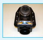
A backwater valve can prevent sewage from an overloaded sewer main from backing up into your basement. The valve is placed directly into the sewer lateral at the foot of your basement wall and will close when there is a sewer backflow. A licensed plumber is essential to ensure proper installation. A valve that is improperly placed could result in a cracked
