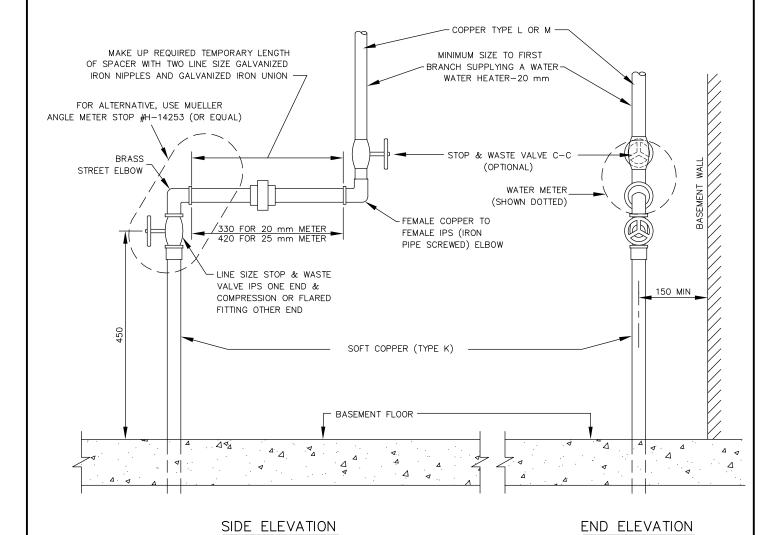
NOTE: METRIC - ALL DIMENSIONS ARE IN MILLIMETRES UNLESS OTHERWISE SHOWN
